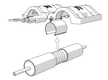
Remove protective paper from EGK and insert cable in inner contact
