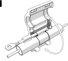
Verify correct position of inner contact in its housings, close plastic
