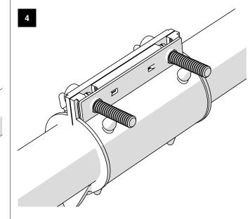
Tightent the screws (3-4 Nm) Done in a few seconds
